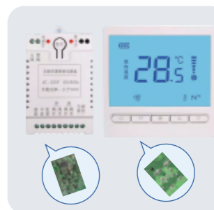
The Cooling/Heating Temperature Control Board
